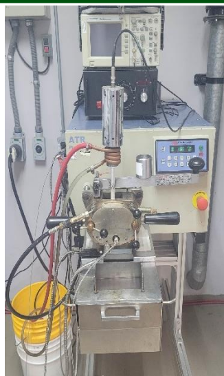
Figure 1. Torque Rheometer equipped with an ultrasonic equipment: sonotrode, generator and converter.
